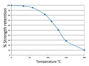
UV625 can withstand higher temperatures for brief periods (such as for paint baking and wave soldering processes) providing the joint is not unduly stressed. The minimum temperature the cured adhesive can be exposed to is -55°C (-67°F) depending on the materials being bonded.
