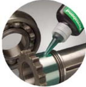
Benefits of using retaining adhesive include rapid, quick and easy assembly of parts. Tolerances can be relaxed, reducing machining times and eliminating the need for interference fits. Adhesive strength is usually higher than alternative methods of fixture. Adhesives have a better fatigue life as they prevent metal fretting (which can be an issue with interference fits).
