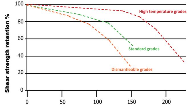
Above: Graph showing how temperature affects strength retention of Permabond anaerobic adhesives.
