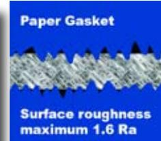
Not only do liquid gasketing adhesives give 100% contact between metal parts, but they also allow the engineer to cut down the amount of surface-finish machining, therefore reducing costs and increasing production rate.
